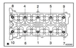
(c) Using a 10 mm bi-hexagon wrench, install and uniformly tighten the 10 cylinder head bolts and plate washers, in several passes, in the sequence shown. Torque: 79 N·m (806 kgf·cm, 58 ft·lbf)
